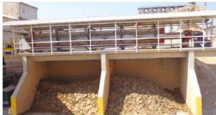
Matec filterpress 100x1300 170 plates
